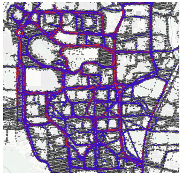
Fig. 2: The density of micromobility travel around the University of Maryland campus. Some of the most frequently traveled edges are shown, with brighter edges representing more frequently travelled paths and the black hexes representing all recorded GPS locations localized to hexes.
